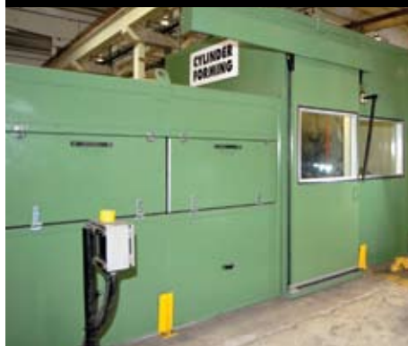
Noisy equipment in the factory has been enclosed, including the power pack for the ultra-large cylinders forge (above) and the forge for forming small cylinder
