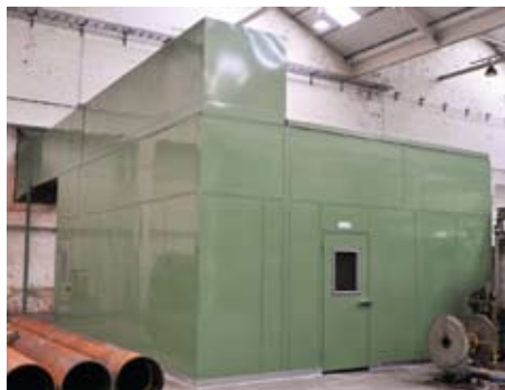
Noisy equipment in the factory has been enclosed, including the power pack for the ultra-large cylinders forge (above) and the forge for forming small cylinder
