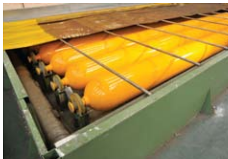
In future, ultra-large cylinders will need to spend less time in these drying cabinets, due to the new paint system being introduced.
