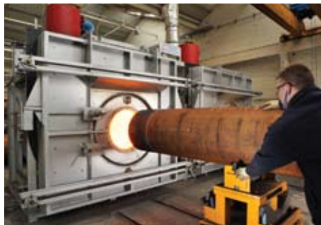
Two new, efficient furnaces have been installed to more rapidly heat tubes ready for forging the necks of ultra-large cylinders.
