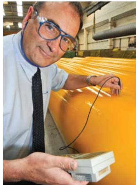
Alan Harding, Quality & Technical Director, has had overall responsibility for achieving ISO 14001. Here he is using a paint thickness monitor on a cylinder freshly painted with the new water-based paint system.
